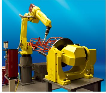
ARC Mate 120iC with coordinated motion on kart frame.
