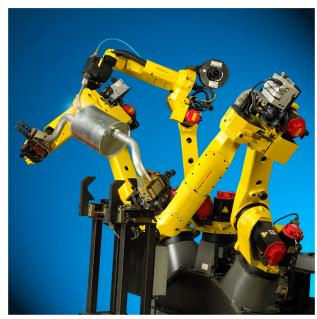
Triple ARM coordinated motion welding exhaust system.
